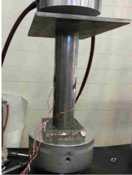
Fig. 4. Testing of steel tube under compressive loading
