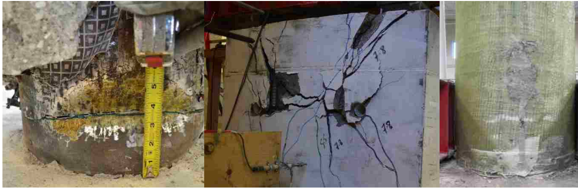
Fig. 8. Columns' modes of failure: (a) steel tube fracture of the F4-24-E325 column, (b) footing damage of the F4-24-E344 column, and (c) FRP rupture of the F4-24-P124-R column
