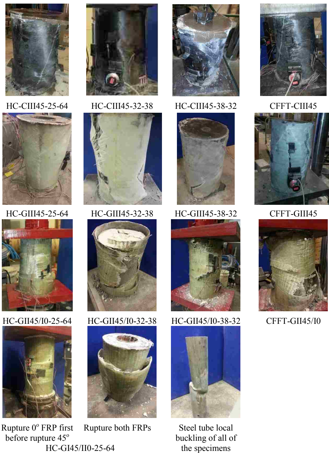
Fig. 13. Modes of failure of all of the specimens and their steel tube local buckling
